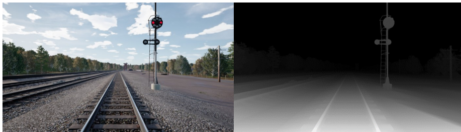
Figure 6.1: RGB image and extracted depth map.
