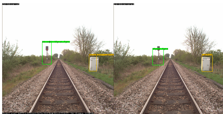
Figure D.3: Example of 2D bounding boxes predictions by the SMOKE model. The left image shows ground truth and right image the prediction.
