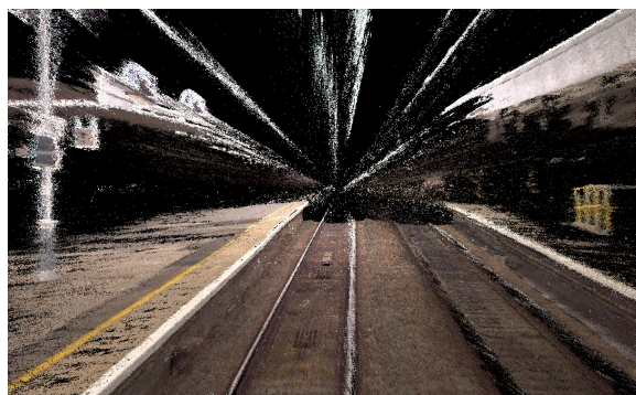
Figure C.7: Incorrectly reconstructed points in SfM point cloud due to features around the center of the image detected incorrectly.
