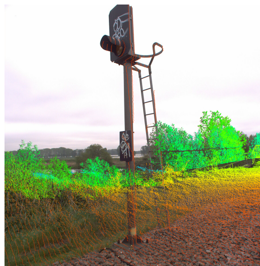
Figure 2.2: Points from laser scanner projected on camera data, showing an object only partially present in the point cloud.
