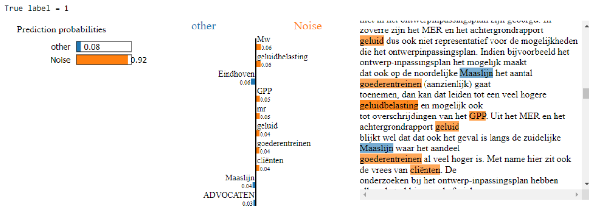
Figure 7: A visualisation of the decision of a Naive Bayes model trained on the category Noise using LIME. The image shows the prediction probabilities for each class, the features that had the most influence on the probability score of the different classes, and the original text with the influential words highlighted in orange for the noise class and blue for the non-noise class.
