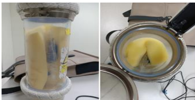
Figure 6: This figure shows the infusion bag wrapped in a foam in PTT tube.
