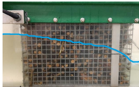
Figure 9. A pressure gradient arises when a viscous fluid flows through a porous medium.
