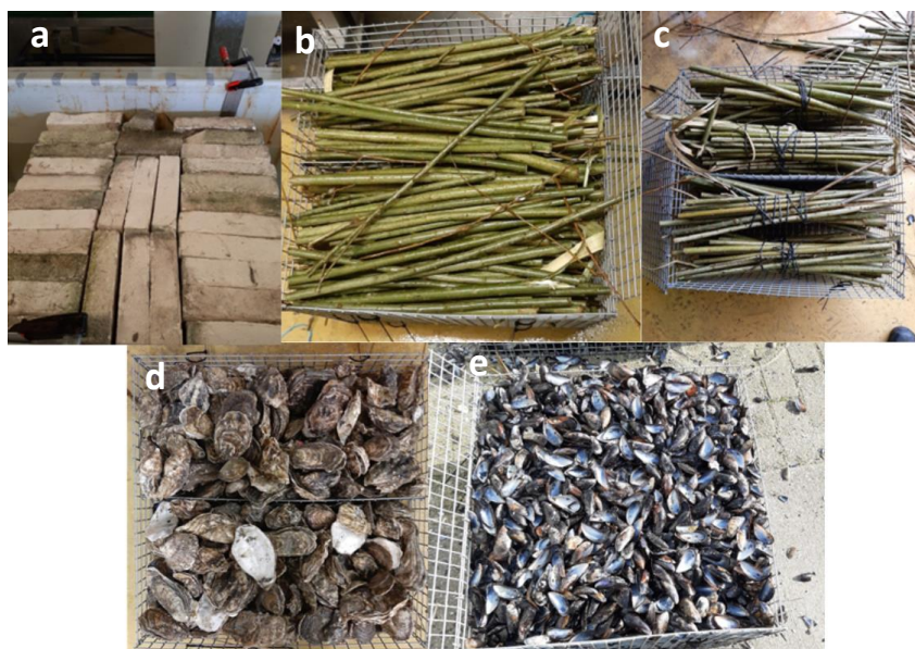
Figure 8. Five different materials were tested in the flume. a) brickstones. b) loose brushwood. c) bundled brushwood. d) oysters. e) mussels
