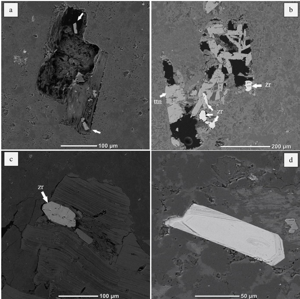
Figure 23: Back-scattered electron (BSE) images of samples analysed under the TTSEM. a) Sample M05101: Iron-oxide inclusions in biotite crystal. b) Sample B07103: Skeletal titanite crystal with zircon inclusions. c) Sample M06101A: Zircon inclusions in biotite crystal. d) Sample 84LTL: Zircon crystal with concentric zoning pattern.
