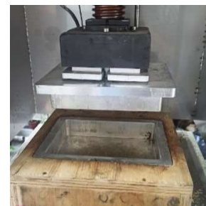
Figure 6: Mould used for pressing experiments.
