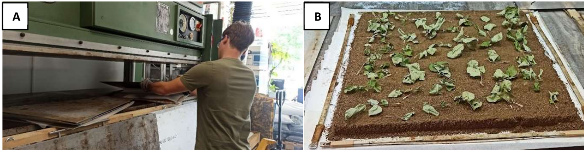
Figure 8: (A) Circlefieds OTT Stabil 2511 veneer press. (B) The flower board just before pressing, the aluminium slats determined the thickness of the board.
