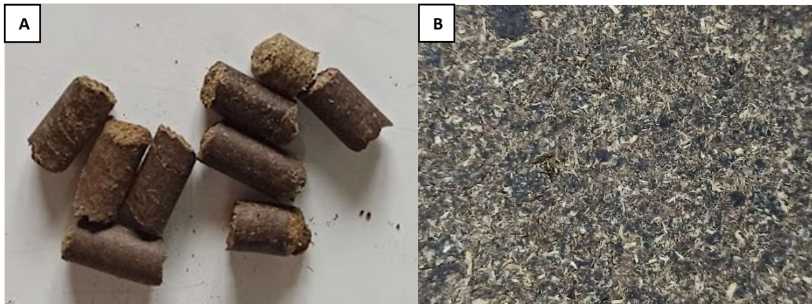
Figure 10: (A) 0.5 mm rose pellets, the raw material used for the boards. (B) close up of 200 g of 0.5 mm rose particles pressed into a board.
