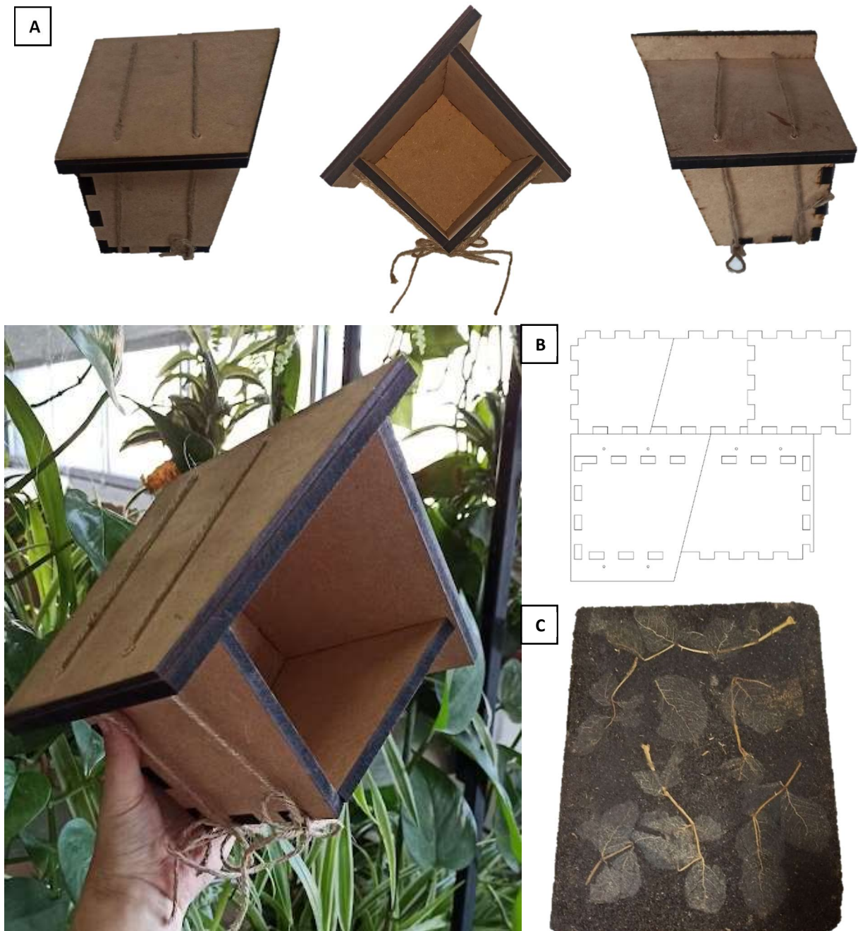
Figure 35: Final prototype design (A) Prototype out of MDF. (B) Laser cutting file. (C) Coated flowerboard which will be the building material.
