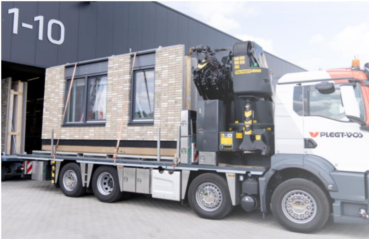
Figure 32 Plegt Vos prefab TFC elements ready for transport from the Plegt Vos
