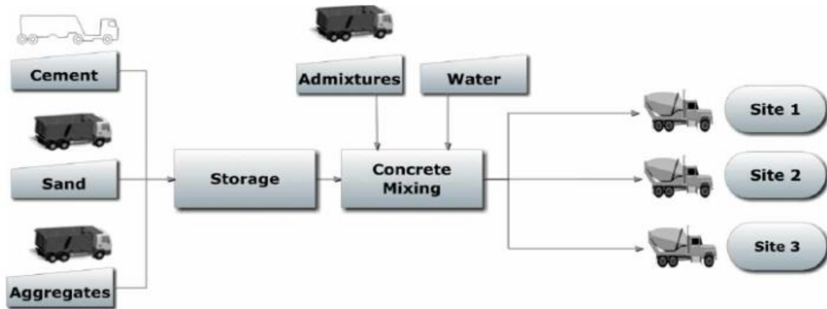
Figure 41 Production process of concrete from cement, water and a combination of chemically inert materials as aggregates such as sand, gravel, crushed stones or recycled (crushed) concrete Source: Chrysostomou et al., 2015
