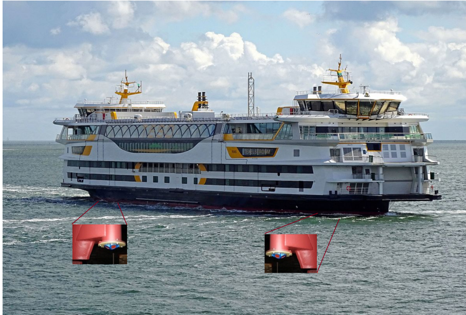
FIGURE 2.1: The TESO ferry sails in the Marsdiep inlet, between Texel and Den Helder. Two ADCPs are mounted underneath the hull below the water surface, toward the bow and the stern of the ferry. The ADCP which is placed on the side of the Texel is denoted tx , while the other one which is placed on the side of the Den Helder is denoted hd . The figure is retrieved from the website of the Royal Netherlands Institute for Sea Research (link: https://www.nioz.nl/en/expertise/wadden-delta-research-centre/facilities-technology/instruments/dynamics-of-the-marsdiep ).
