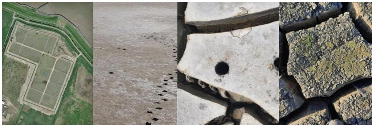
Figure 4 Sediment ripening. The first picture from the left shows an aerial view of the sediment ripening reservoirs. Sediment ripening over the duration of 3 months is shown in the other three pictures from left to right. Pictures from Martine et al. (2021)
