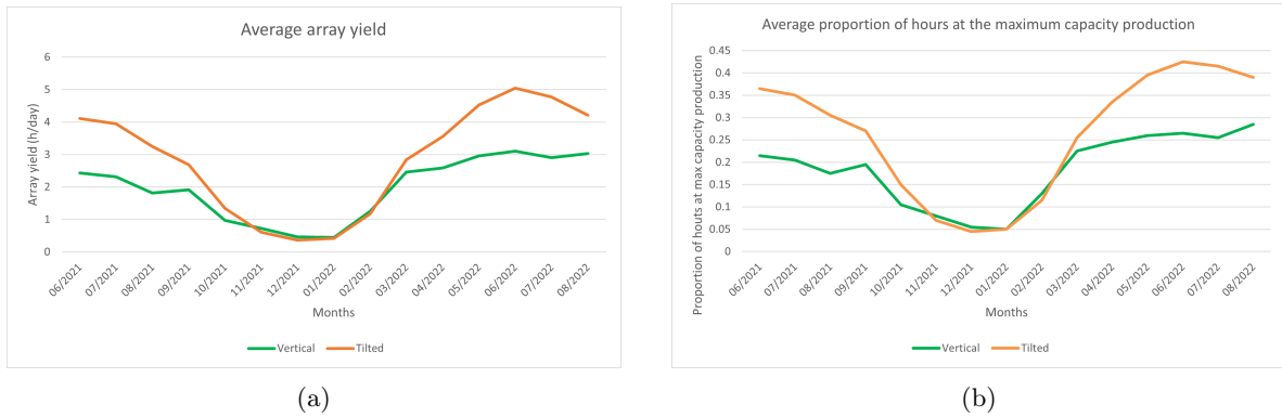
Figure 54: Average array yield (h/day) (a) and proportion of hours in which energy is produced at installed capacity over the total hours of energy production (b) comparison for vertical and tilted modules on the pergola.
