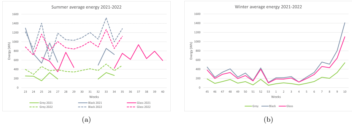
Figure 60: Average energy production (Wh) comparison of grey, black and glass modules, divided into summer (a) and winter (b).
