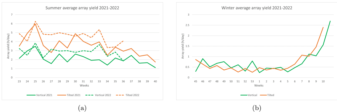
Figure 48: Average array yield (h/day) comparison of modules positioned on pergola vertical and tilted, divided into summer (a) and winter (b).
