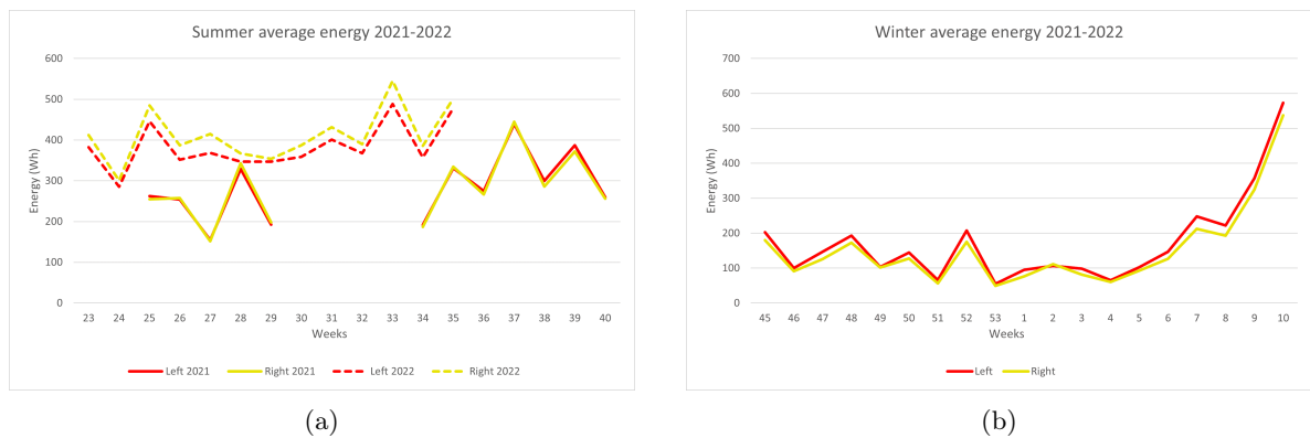
Figure 25: Average energy production (Wh) comparison of modules positioned on the left and right of balconies, divided into summer (a) and winter (b).
