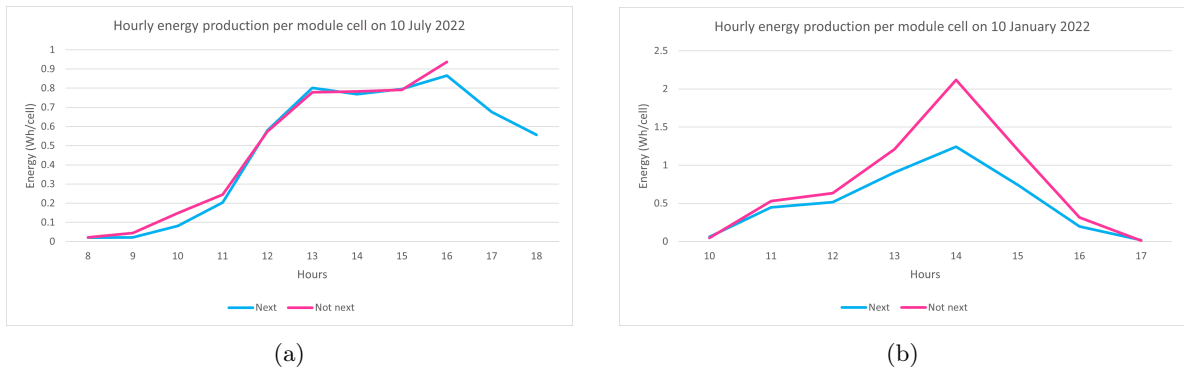
Figure 42: Hourly energy production per module cell, for three modules of which two are positioned next to a balcony and the third one distant from it, during summer (a) and winter (b).
