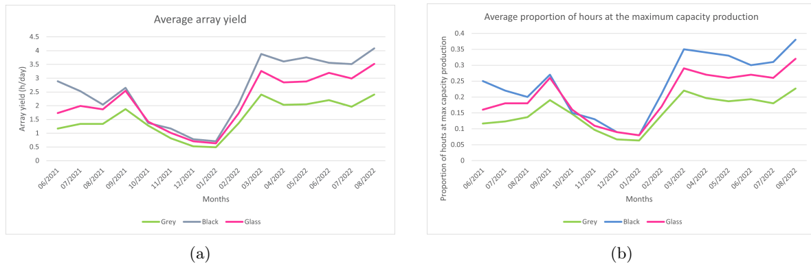
Figure 64: Average array yield ( h/day ) (a) and proportion of hours in which energy is produced at installed capacity over the total hours of energy production (b) comparison of grey, black and glass modules.
