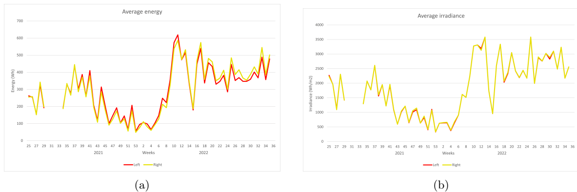
Figure 34: Average energy production (Wh) (a) and irradiance (Wh/m 2 ) (b) comparison of modules positioned on the left and right of balconies.
