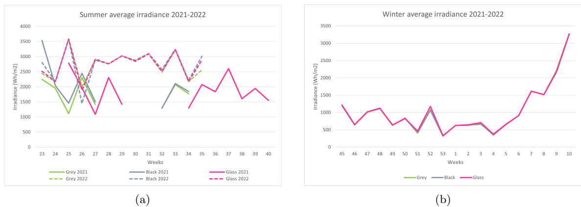
Figure 61: Average irradiance (Wh/m 2 ) comparison of grey, black and glass modules, divided into summer (a) and winter (b).
