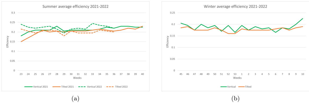
Figure 47: Average efficiency comparison of modules positioned on pergola vertical and tilted, divided into summer (a) and winter (b).
