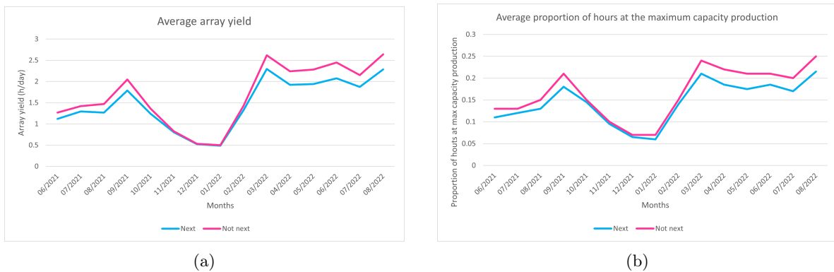
Figure 44: Average array yield (h/day) (a) and proportion of hours in which energy is produced at installed capacity over the total hours of energy production (b) comparison for modules next to balconies and not next to balconies.
