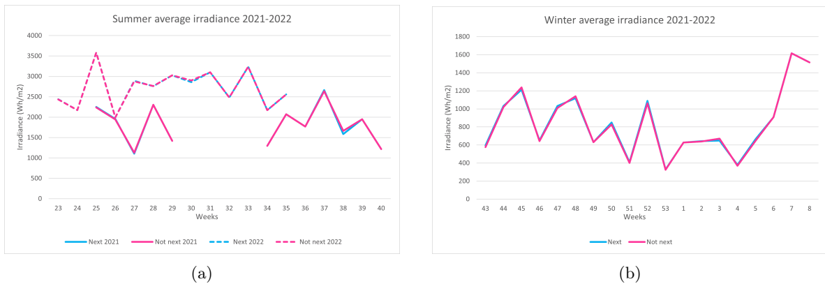
Figure 39: Average irradiance (Wh/m 2 ) comparison of modules positioned on the façade next to balconies and not, divided into summer (a) and winter (b).
