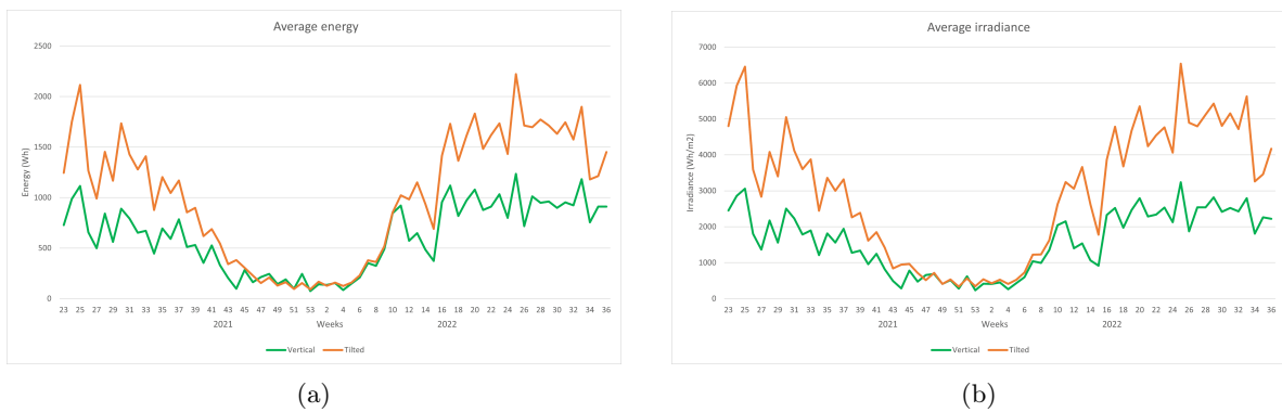
Figure 55: Average energy production (Wh) (a) and irradiance (Wh/m 2 ) (b) comparison of modules positioned on pergola vertical and tilted.
