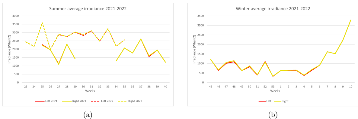
Figure 26: Average irradiance (Wh/m 2 ) comparison of modules positioned on the left and right of balconies, divided into summer (a) and winter (b).
