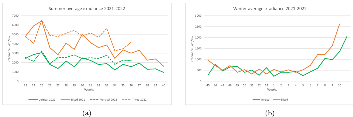
Figure 50: Average irradiance (Wh/m 2 ) comparison of modules positioned on pergola vertical and tilted, divided into summer (a) and winter (b).
