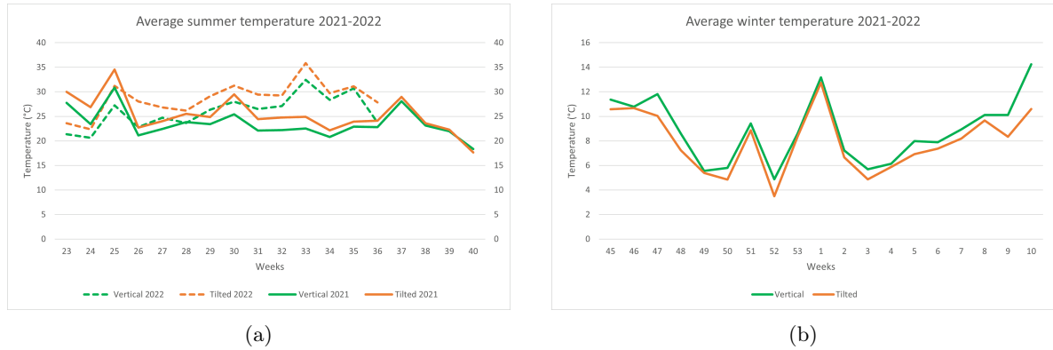
Figure 51: Average temperature comparison of modules positioned on pergola vertical and tilted, divided into summer (a) and winter (b).
