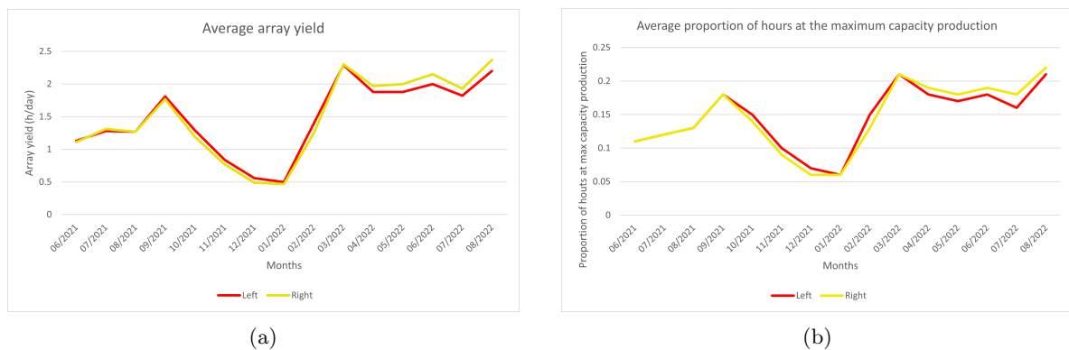
Figure 33: Average array yield (h/day) (a) and proportion of hours in which energy is produced at installed capacity over the total hours of energy production (b) comparison of modules positioned on the left and right of balconies.
