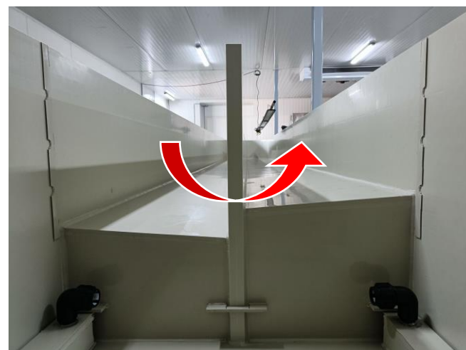
Figure 3: Picture from inside an empty TinyOcean, taken from the purification part (front region), with at the left side a deeper water column than the shallower right side. The red arrow indicates the designed flow direction. The flume is slowly descending to the middle wall as well, extra stimulating the sediment to end up on the seabed.
