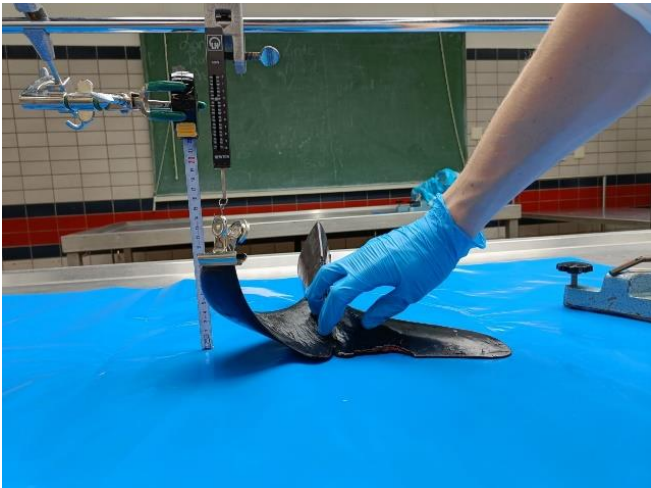
Figure 12: The setup of the stiffness experiment with a real harbour porpoise fluke, using a force meter (Newton).
