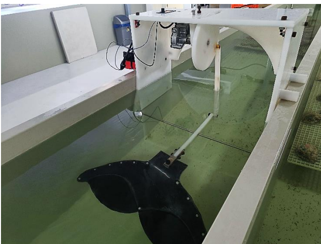
Figure 29: The large fin inspired by the gray whale ( Eschrichtius robustus ) at 50% motor power comes out as the most efficient option based on the experiments conducted in this project.
