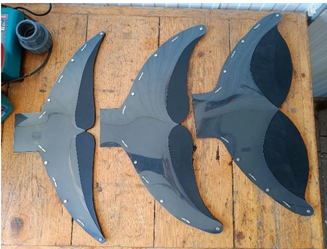
Figure 13: The reinforced prototypes with two specifically shaped layers of 0.8 mm polyethylene (light grey colour in this picture) added to each fin, making each fin 5.6 mm thick.
