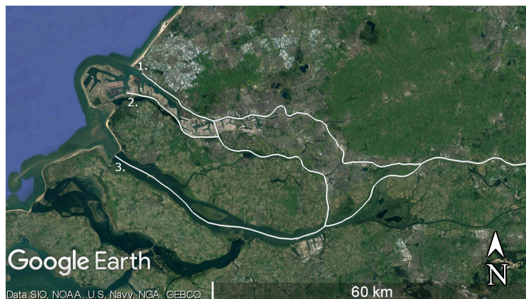
Figure 1.3: Satellite image of the Rhine-Meuse estuarine network. The white lines are the channels considered in this study. The tidal wave enters the Rhine-Meuse at position 1. (Nieuwe Waterweg) and 2. (Hartelkanaal). At position 3. (Haringvliet) a dam and several sluices are located that close during flood and open during ebb. Source: Google Earth.
