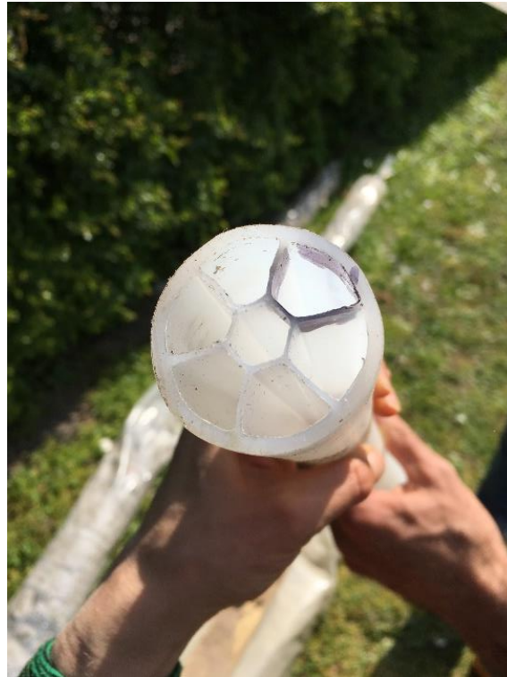
Figure 9: Multi-Level Sampler with 7 channels installed in the Griftpark subsurface.
