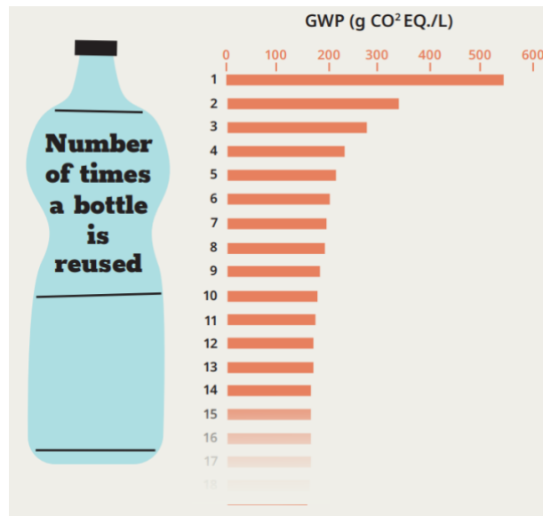
Figure 4: Number of trips and the decrease in Global Warming Potential (gCO 2 eq/L) taken from Coelho et al.(2020b)
