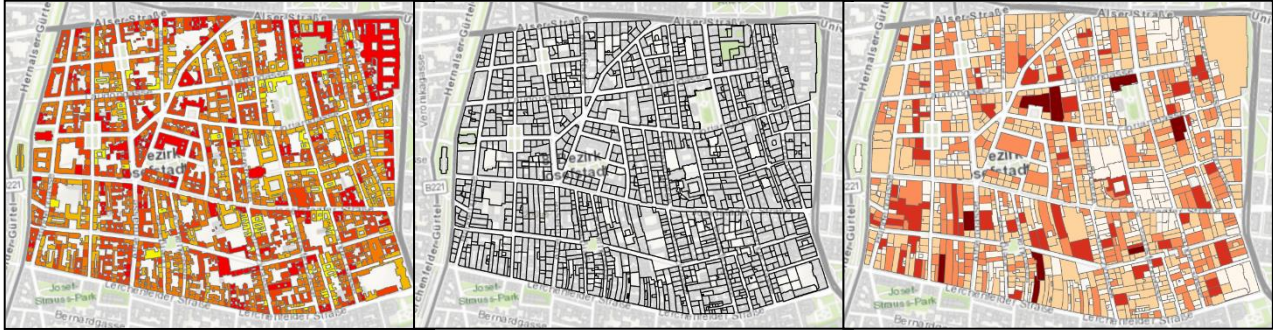
Figure 8: From left to right (1) building footprints with height information; (2) land register parcels; (3) spatially joined datasets with calculated FAR, where darker colors mark higher values
