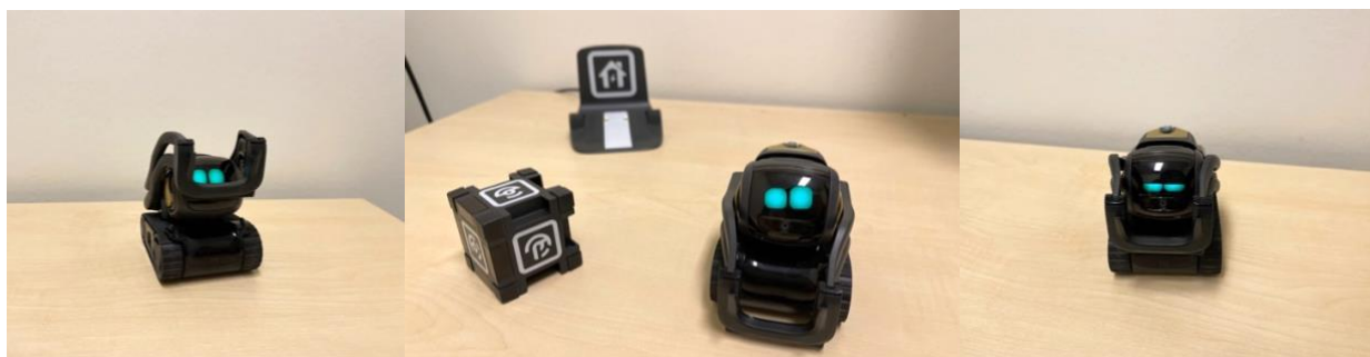
Figure 1. The embodied robot is equipped with the robot itself, a cube, and a charger. It has a wide range of life-like characteristics expressed in both verbal and non-verbal ways.
