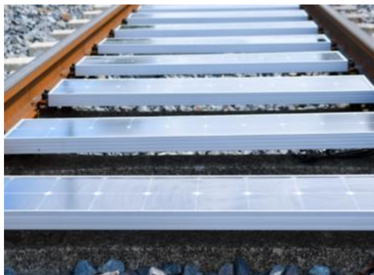
Figure 14: Tests of small PV panels in between the rails by Deutsche Bahn & Bankset Energy in Germany (Seijlhouwer, 2022)
