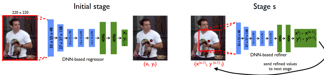
Figure 1. The architecture of the DeepPose model, only layers with parameters are visible (Toshev and Szegedy, 2014).
