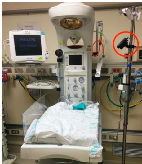
Figure 2.2: Example of an unobtrusive set-up for RR monitoring. Camera is highlighted with a red circle. Image was retrieved from Rossol et. al. [24].
