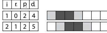
Figure 5.1: Example of two activities on the same machine. The light grey tiles denote when the activities can be executed and the dark grey tiles denote the processing times.
