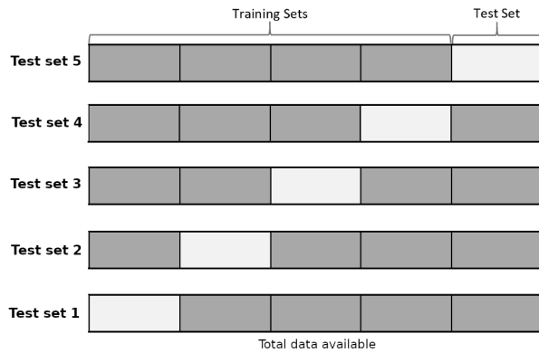
Figure 3: Representation of the five different test-train splits from the available data used to evaluate the models, with time increasing from left to right.
