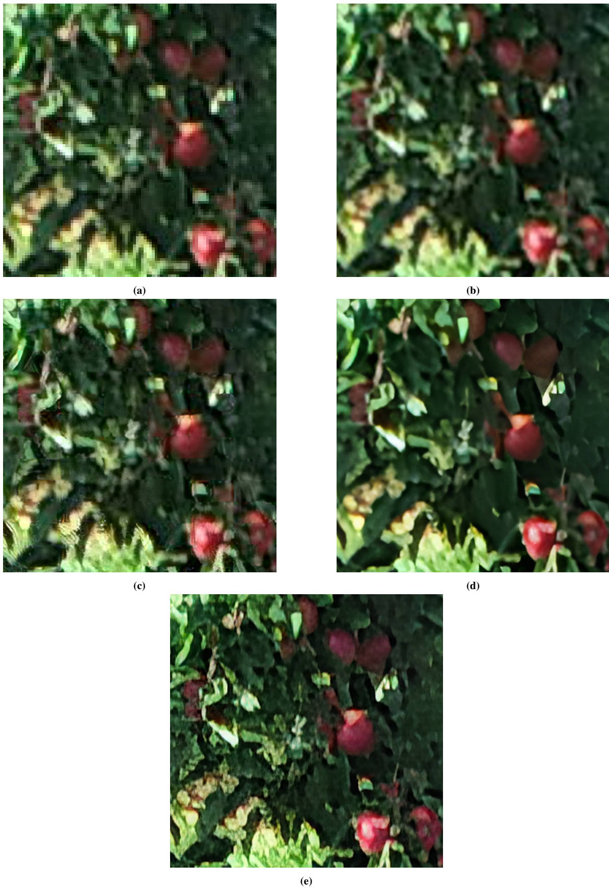
Figure 4.1: Example of super-resolution (SR) reconstructions of the (a) original dataset: (b) Bicubic Interpolation, (c) ESRGAN, (d) Real-ESRGAN not fine-tuned in the dataset, and (e) the domain-specific Real-ESRGAN fine-tuned using a limited number of UAV imagery
