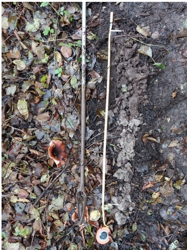
Figure B.1.8: Soil profile at location 2, topsoil at plopper/dompelklokje instead of auger handle
