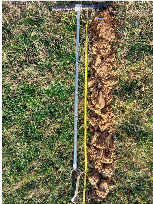
Figure 14: Soil profile from excavated part of location 8.
