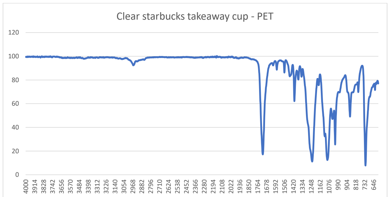
Figure 44: IR spectrum Starbucks takeaway cup. The peaks at around 1750\text{-}1735\text{ cm}^{-1} denote C=O bonds in Esters
