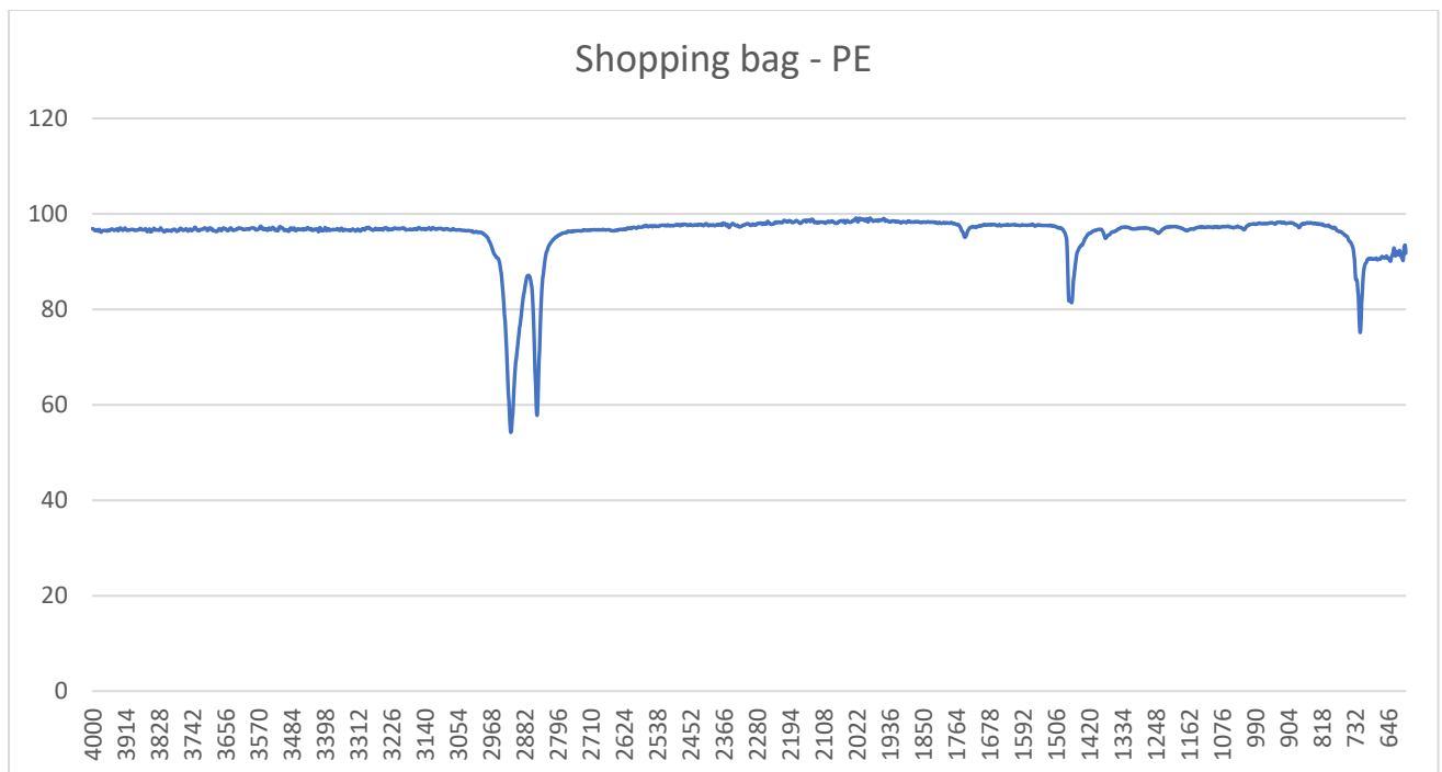
Figure 45: IR spectrum of a shopping bag. The peaks around 2917, 2850 and 718 \text{cm}^{-1} help to point towards PE, mostly likely LDPE.
