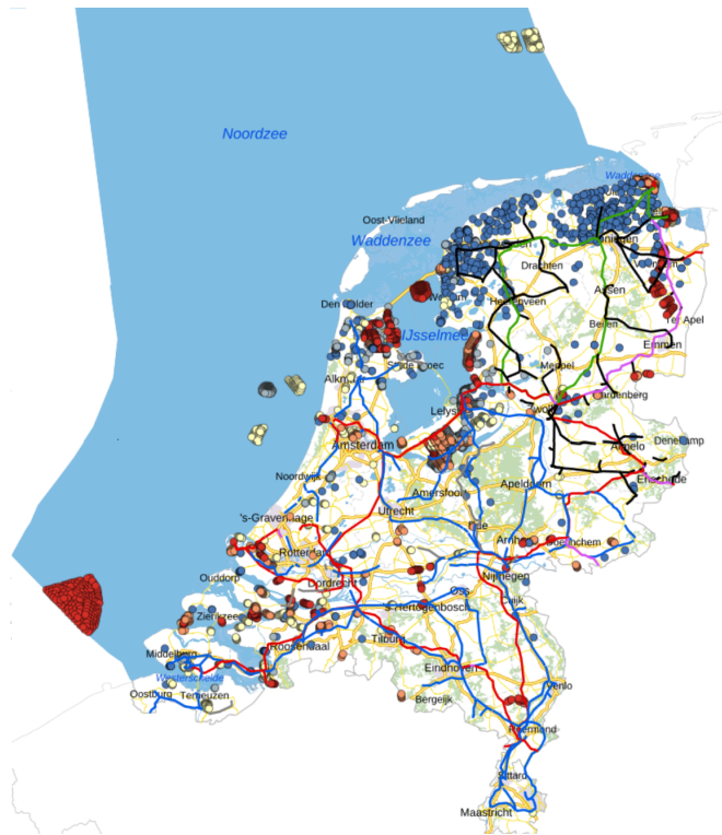
Figure 2: Location of wind turbines (dots, all colours) in the Netherlands, at February 22, 2022. The lines represent the high voltage transmission network. Transmission voltages included are: 380kV (red), 220 kV (green), combi line (pink), 150 kV (blue), 110 kV (black) and 50 kV (grey). Figure adapted from Atlasomgeving (2022).
