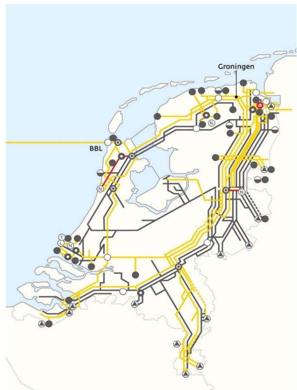
Figure 15: Transmission network operated by Gasunie in the Netherlands.
