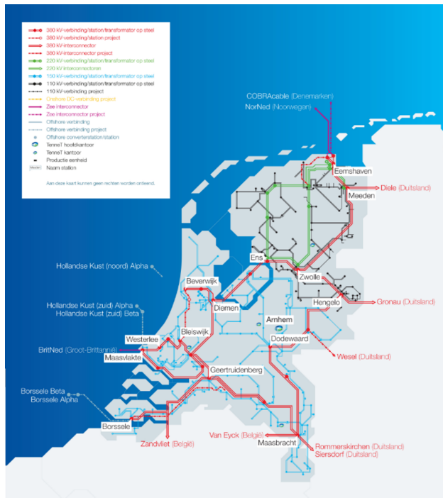
Figure 14: High voltage transmission network operated by TenneT in the Netherlands.
