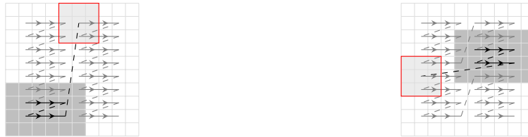
(a) Grouping by column only incurs a heavy load every time a new column is started.
