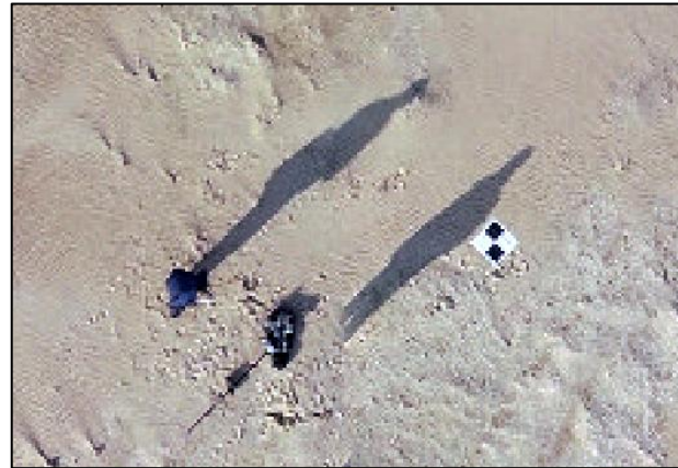
Figure 13: A GCP (black and white square) visible in the final orthophoto, together with the UAV operators. The real dimensions of the GCP are 50 by 50 cm.
