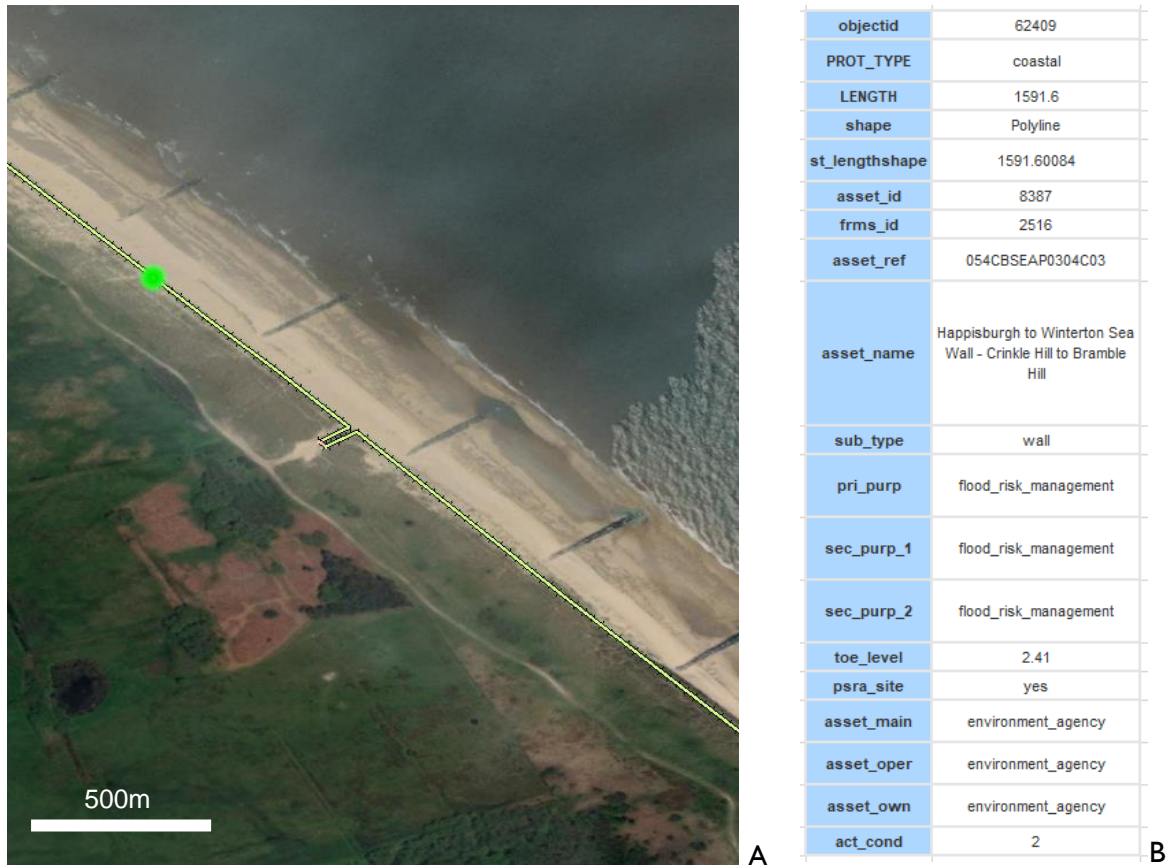
Environment Agency AIMS – Winterton-on-Sea, Norfolk, UK - A) Feature Layer, B) Item Attributes
