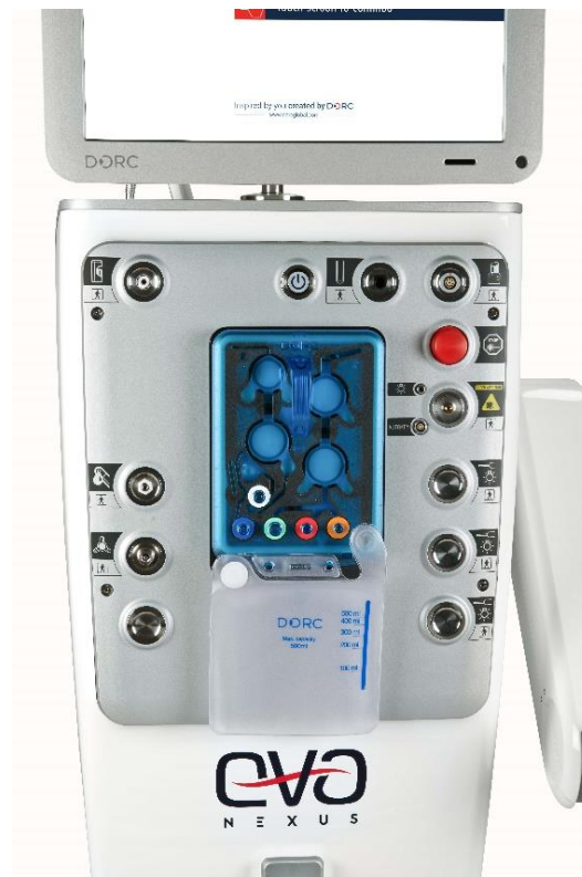
Figure 3 The EVA NEXUS machine with the day-cartridge with waste collection bag (D.O.R.C., n.d.-b)
