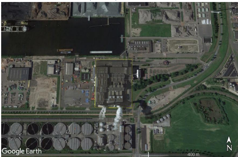
Figure 30. AEB. This is a large waste furnace for the public waste service of the Amsterdam municipality. The location next to the largest WWTP and the curved road structure didn't allow any good transects. Methane enhancements were detected, but the exact source on the terrain could not be estimated.
