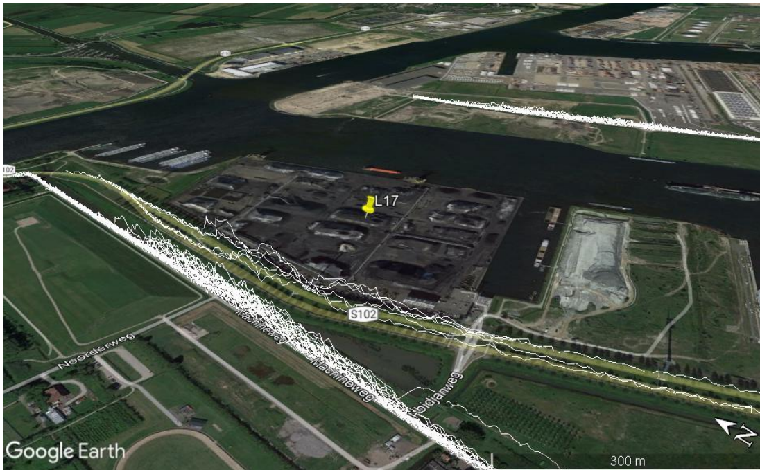
Figure 38. Rietlanden Terminals. The yellow pointer indicates the coordinates of the assumed point source in the middle of the facility. Measurements were done on a close road to the west, a parallel road somewhat further to the west, and a road across the water to the east.
