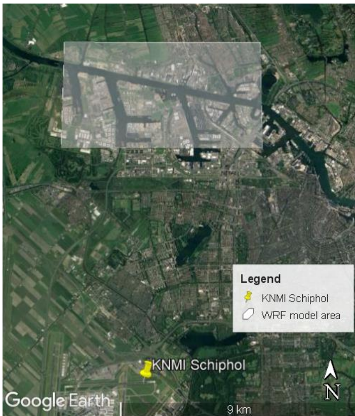
Figure 5. A map of the port of Amsterdam area with the KNMI measurement station at Schiphol roughly 9 km to the south of the port. The white rectangle shows the 52.40^{\circ} - 52.44^{\circ} , 4.74^{\circ} - 4.86^{\circ} area, over which the WRF model results are averaged and used.
