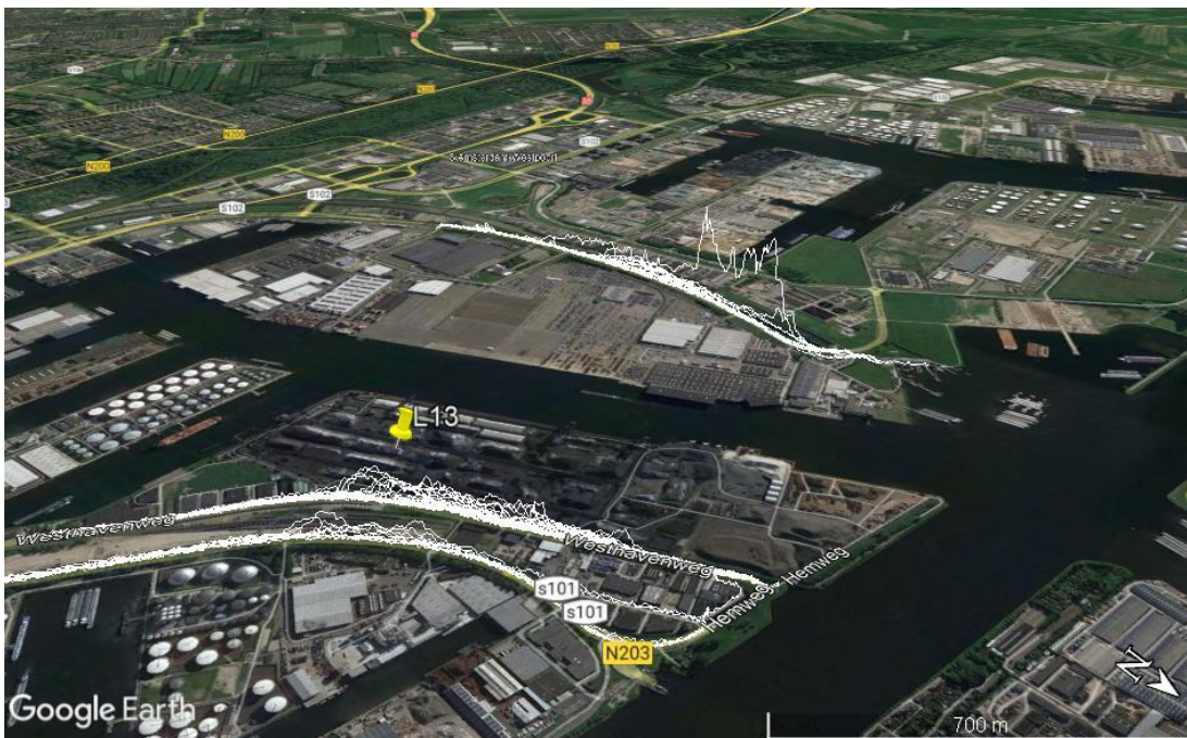
Figure 34. OBA Terminal. This coal transshipment facility extends far in the N-S direction. Therefore, the roads to the east often showed 2 peaks, indicating it is too close for the GDPM. The road to the west is at a larger distance, and the plumes on this road showed better gaussian shapes.
