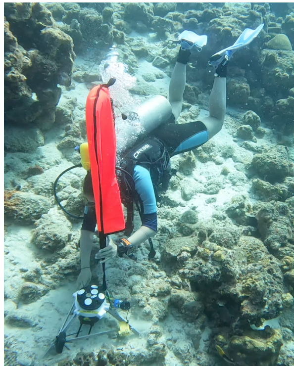
Figure 7: Transportation of the AD2CP and PME miniDOT. The orange dive balloon was attached to the AD2CP frame and oxygen logger via removable clips
