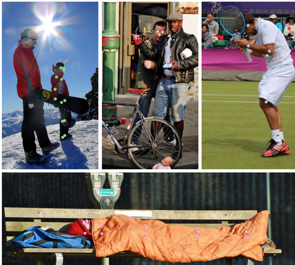
Figure 4.4: Different examples of wrong occlusion labels given to keypoints. Top Left: The snowboard occludes several keypoints, but none are labelled as occluded. Top Middle: The majority of keypoints are labelled as occluded, while most of them are visible. Top Right: The eyes, nose and right wrist are all labelled as occluded while these are visible, but other labels such as the right elbow are corrected as occluded since self occlusion is present. Bottom: Keypoints occluded by a blanket can be thought of as occluded, but also as not occluded. However, most keypoints under blankets were labelled as occluded, hence for the sake of consistency every keypoint under a blanket is corrected as occluded.
