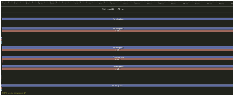
(a) A GC call that caused an extreme 37ms stagnation of the worker threads. This entire iteration took 44.7ms. For reference, most iterations take around 7-13ms, and the GC in the image to the right takes around 1/200th of the time.
