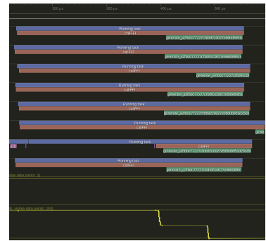
(b) A GC call that caused almost no stagnation of the worker threads; the waiting time is around 200 \mu s.
