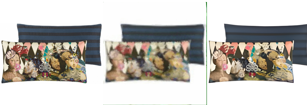
FIGURE 4.7: A comparison on an image of the Interior category. From left to right: The ground truth, x8 upscaling by SDMD (MS-SSIM 0.794, PSNR 17.372) and the x4x2 upsampled image (0.882, 20.828). When zooming in it can be seen both models struggle with the amount of detail in the ground truth image, most probably due to the small size the ground truth image has when downsampled.
