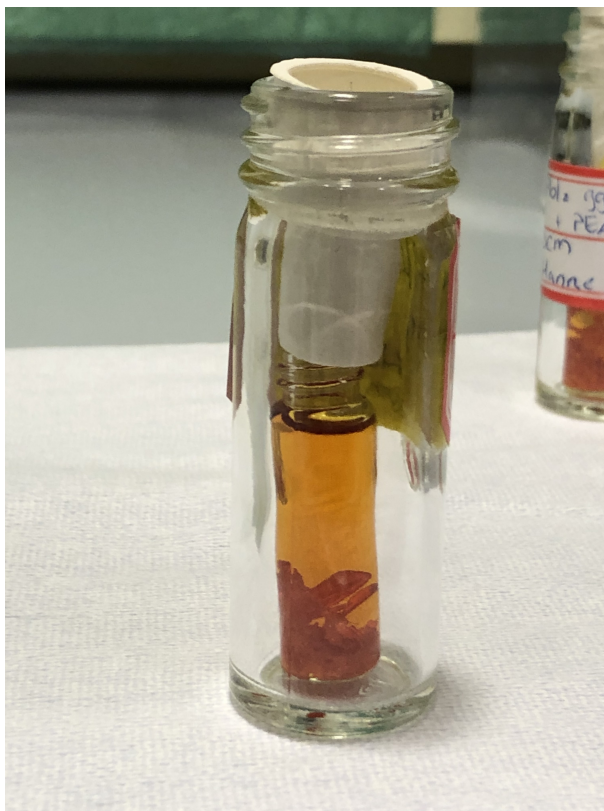
Figure 3: The set-up after a crystallization period of five days. The antisolvent has diffused into the smaller vial and dark-orange crystals have formed inside the small vial.
