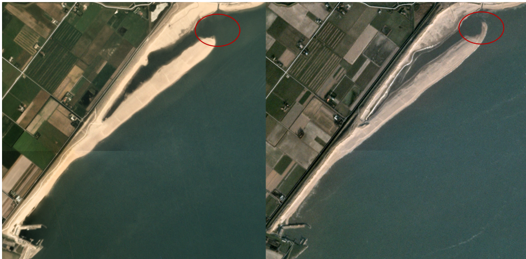
Figure 32: Longshore development over 2.5 years. Left: July 2019. Right: December 2021.
