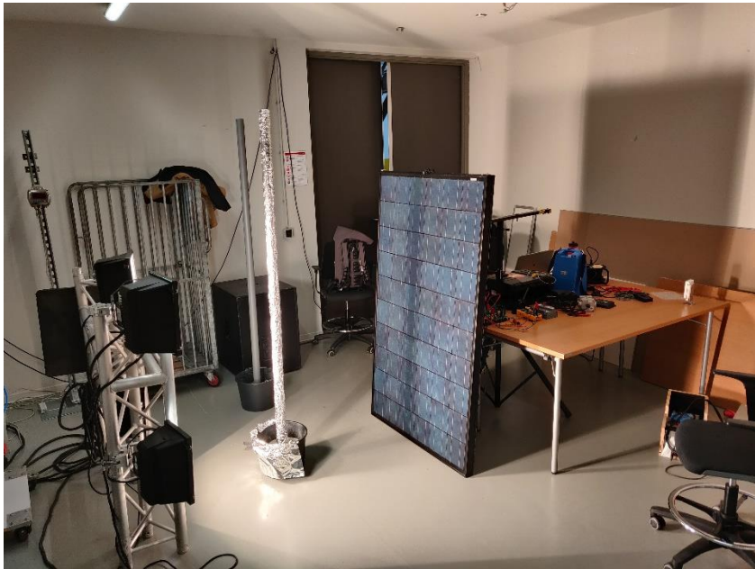
Figure 1: Smart PV panel setup with construction lamps for light.
