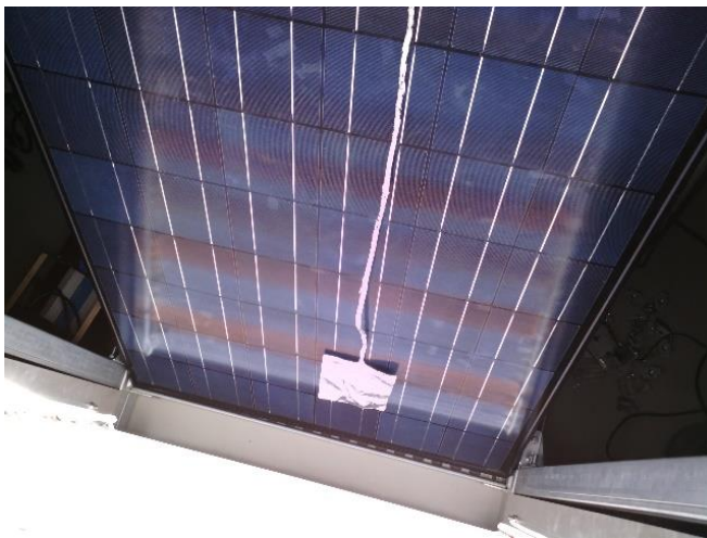
Figure 3: Example of the object for creation of shadow on the PV panel. In the figure it is hanging on against the panel during one of the test rounds.
