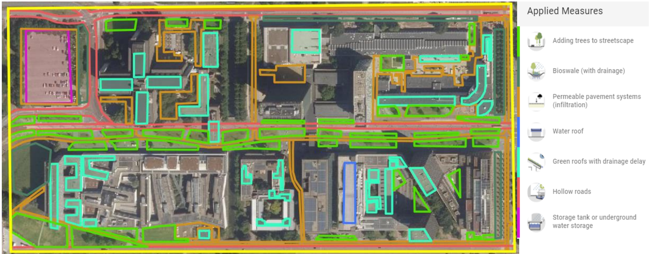
Figure 32: Climate adaptation strategies that could be applied to the Centrumgebied to address both heat stress and pluvial flooding risk. This map was created based on the current land-use of the centrumgebied. Measures were applied to retain the function of each area, but alter it in such a way to be more climate adaptive based on the hazard type and risk level (Figures 31). For example, the grassy vegetation has all been replaced by trees. Walkways and cycle paths have been replaced by permeable pavement systems. Roads and tramways have been fitted with hollow roads.
