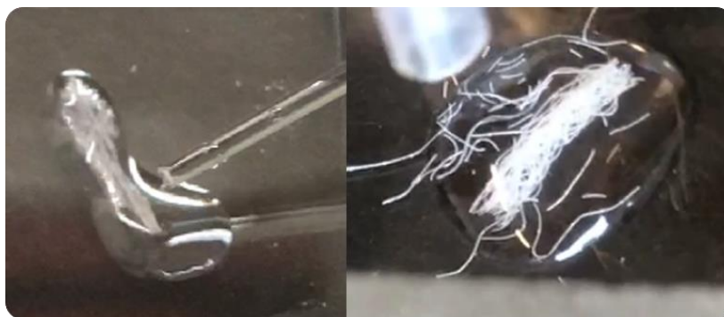
Figure 15: Water droplets were introduced to HTES-treated fibers to probe their wettability. Contrary to expectation, the droplet completely covered the fiber, which indicated a hydrophilic character.
