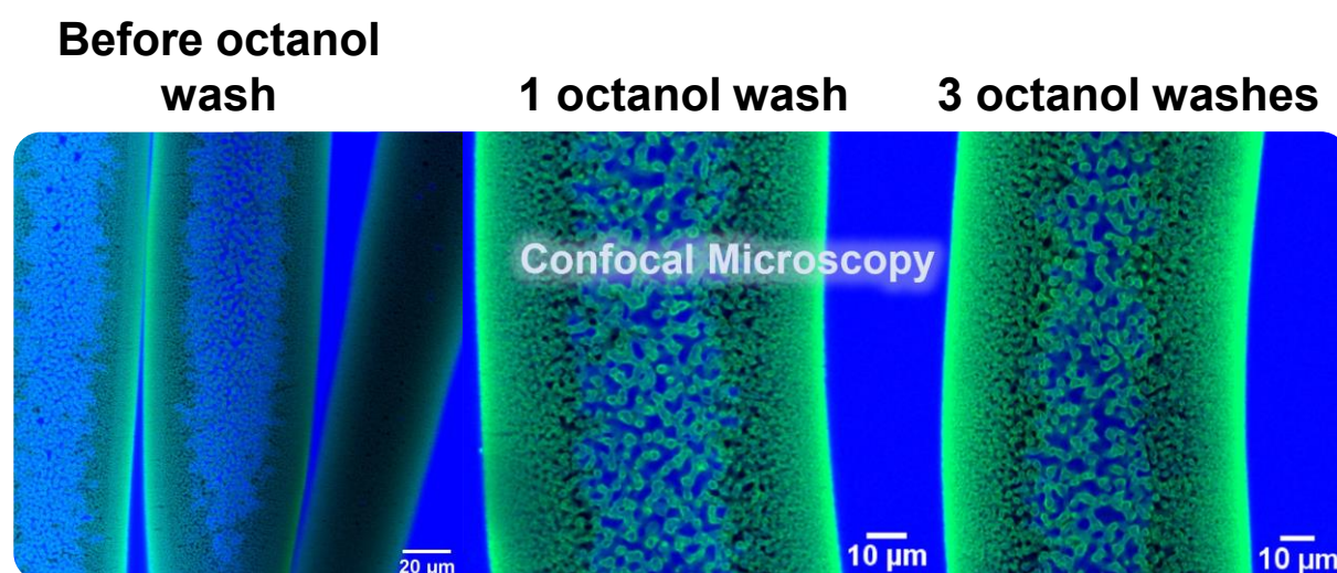
Figure 19: Confocal micrographs of octanol-washed fibers which show hexane-to-water channel leakage. Mineral oil was the solvent during TEOS-treatment.
