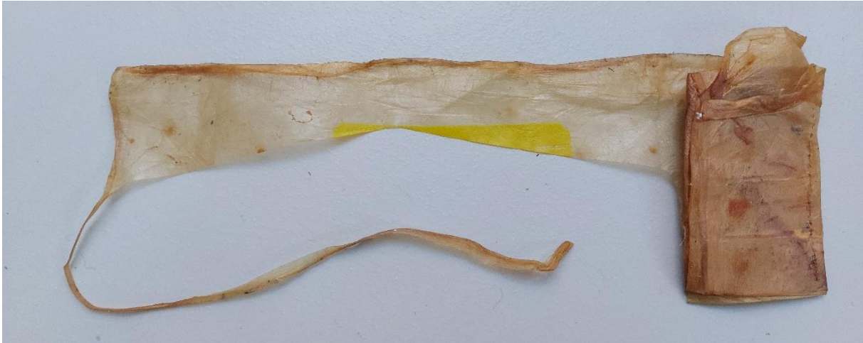
Figure 5: Kombucha-derived cellulose. From a bundle of cellulose layers on the right, a single sheet of cellulose is rolled out to the left.
