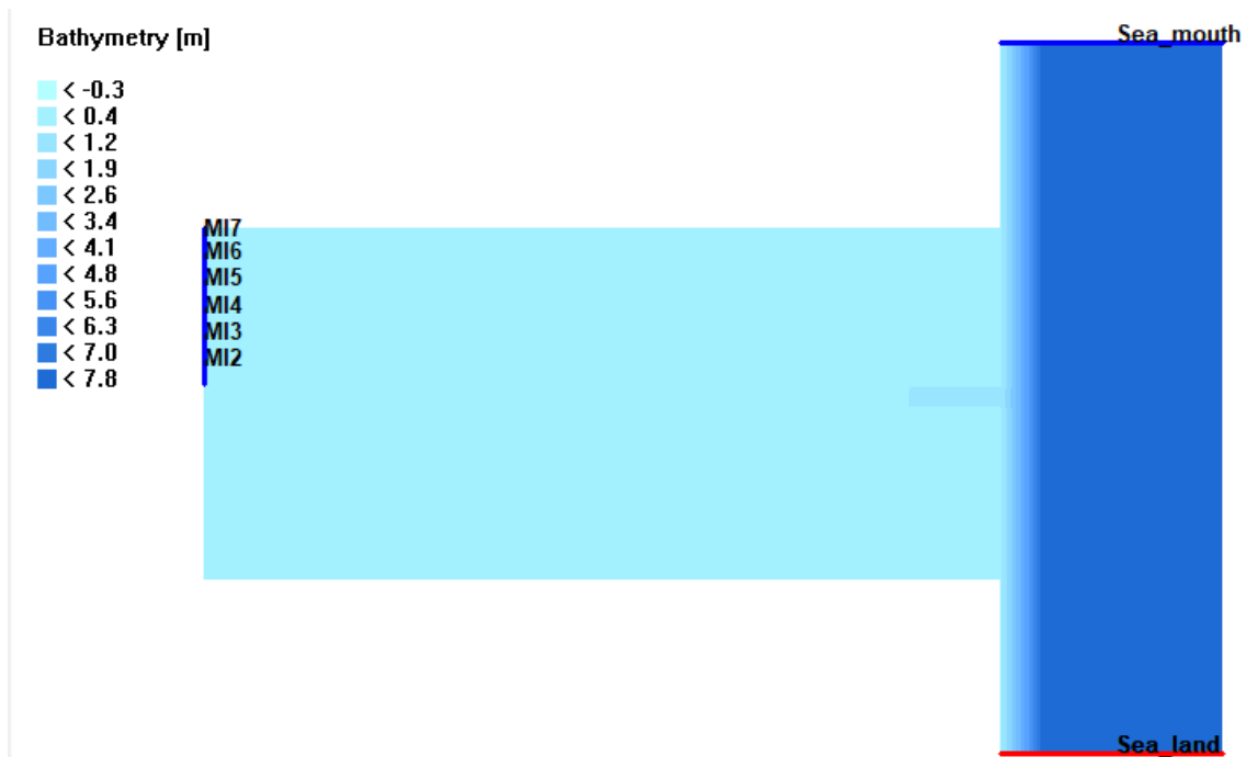
Figure 26: Bathymetry of the basin as computed from a MATLAB code. This T-shaped boundary has two open boundaries on each side of the ocean basin each implementing a harmonic signal on the ocean basin with only 4 minutes difference. The mud-inflow boundary is the open boundary up onto the tidal flat. Through this boundary, the mud is added to the system.
