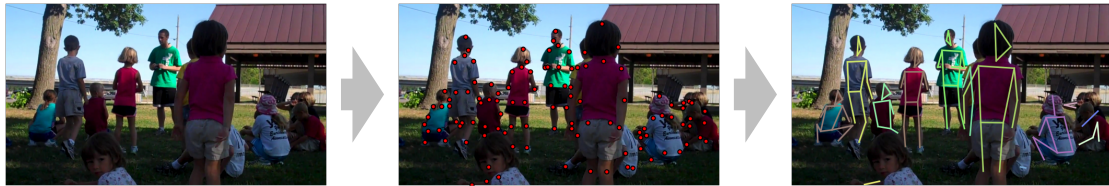
(b) With a Bottom-up approach, all visible joints are detected at once, which are then used to construct the most probable skeletons.
