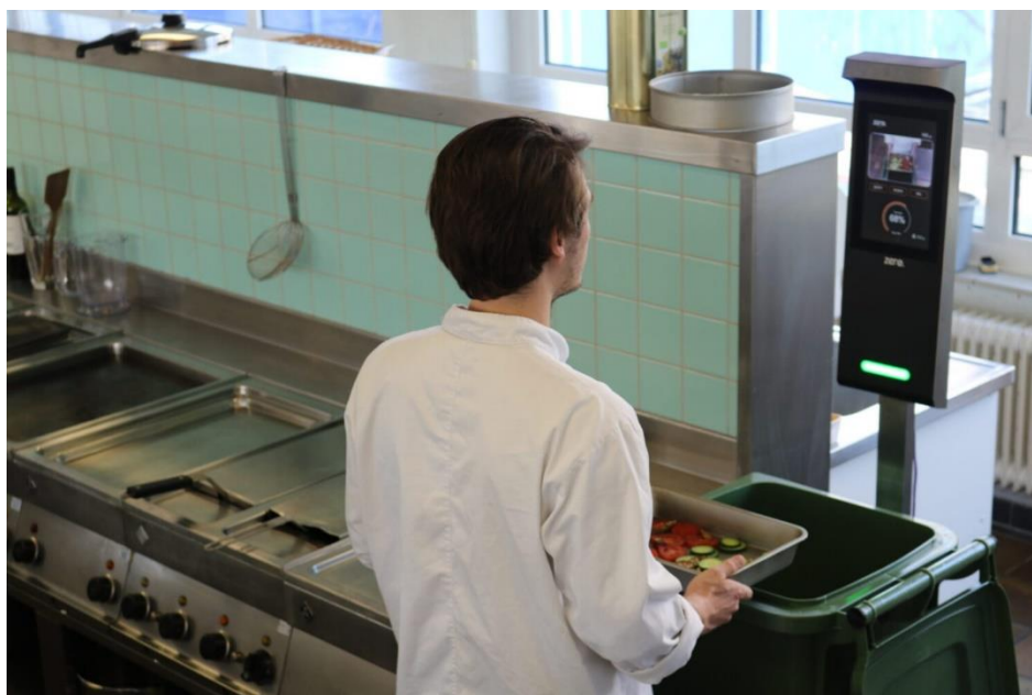
Figure 3: Orbisk Hardware system (from Orbisk.com)
