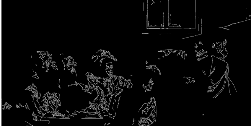
Figure 2.4: The edges of “The Calling of Saint Matthew” calculated by the Canny Edge Detector.
