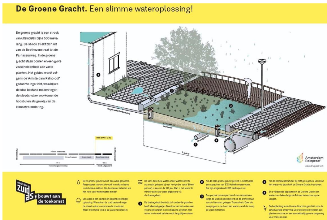
Figure 13: Project sign of the Green Strip at Prinses Irenestraat (Zuidas and Amsterdam Rainproof).
