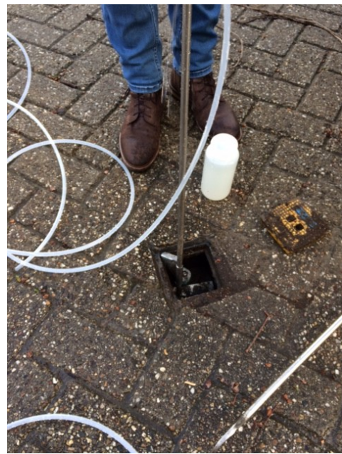
(b) Groundwater level measuring well.
