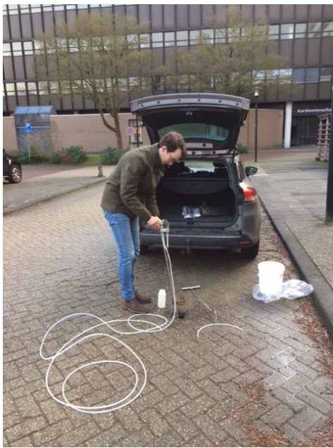
(a) Extracting groundwater.
