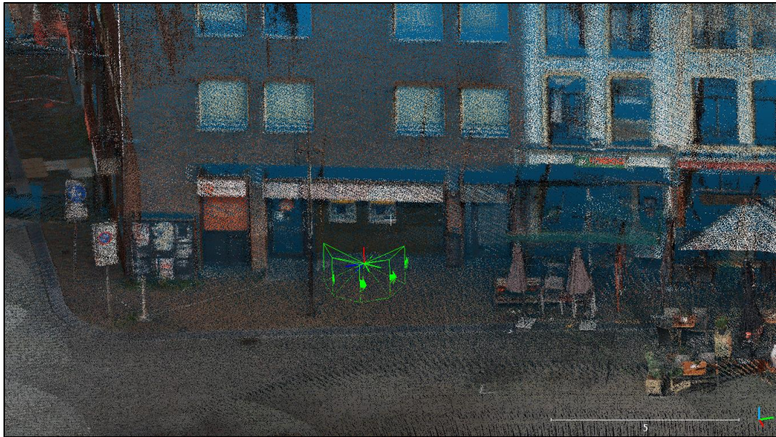
Figure 6.4: The 4 definite cameras used in the HPR analysis, providing an undistorted view of 180 degrees around the ATM
