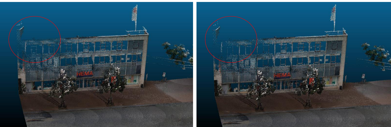
Figure 3.10: On the left image there is no noise removal and on the right image there is noise removal. The red circle shows that the façade of the building partly vanishes due to the noise removal (Cyclomedia, 2020)
