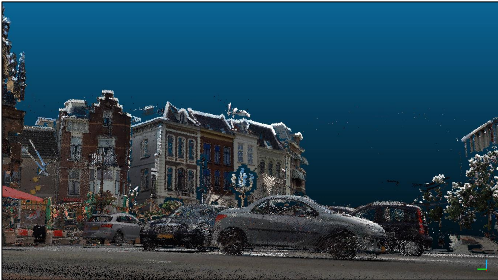
Figure 6.7: The perspective from camera 3 with HPR, octree level 7, applied onto it and an increased size in points, which improves the visibility
