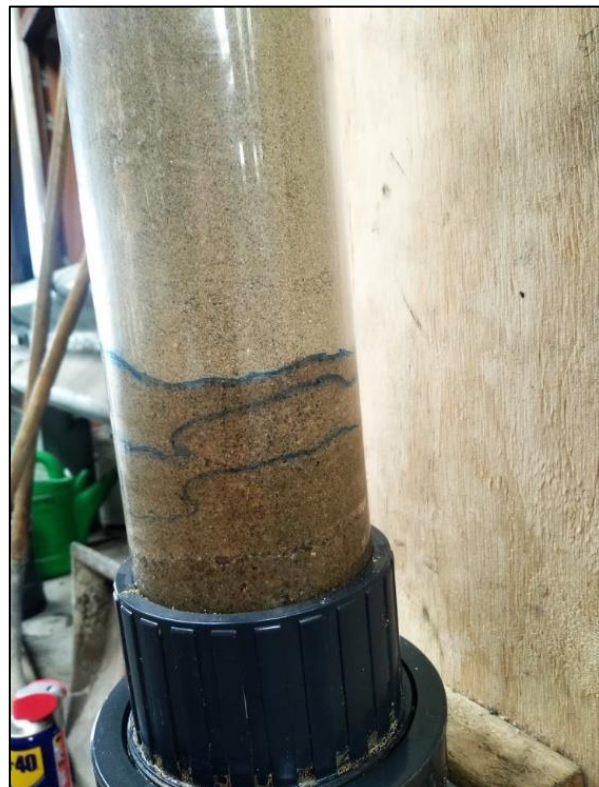
Figure 3.5. An overview of the saturating sand column. The blue markings indicated saturation levels 30 minutes apart. The bottom line represents t=0.3
