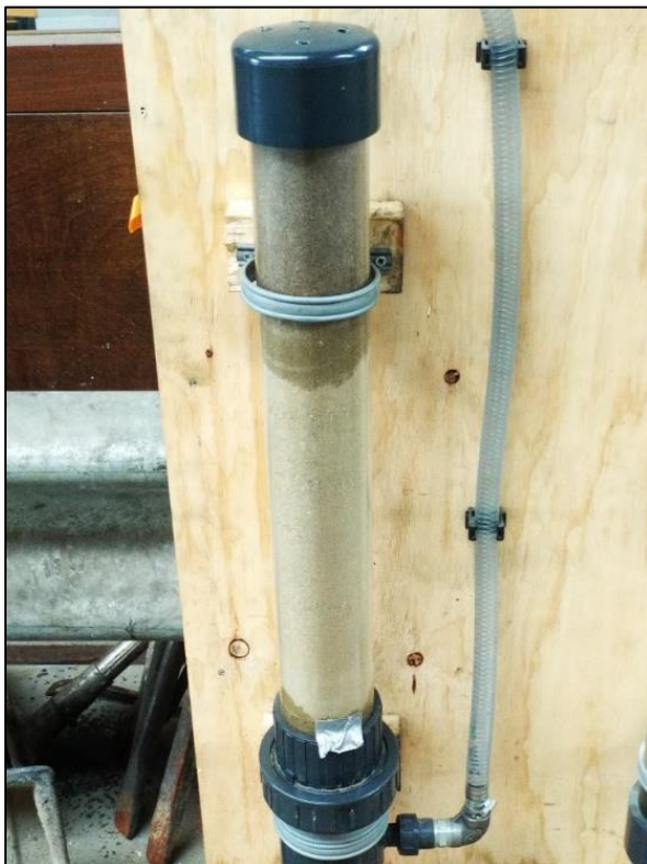
Figure 3.5.2 The gravity permeation grouting sample. First dry sand was added, and then semi saturated sand was added on top.
