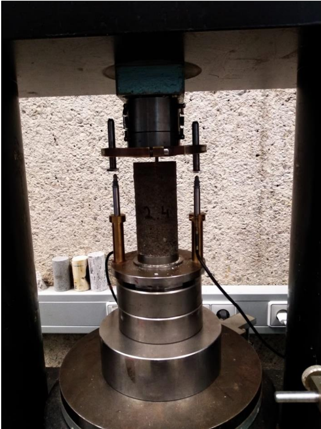
Figure 3.5.4 The device used in the UCS experiments. The red markings demonstrate the metal plates that enclose the sample.
