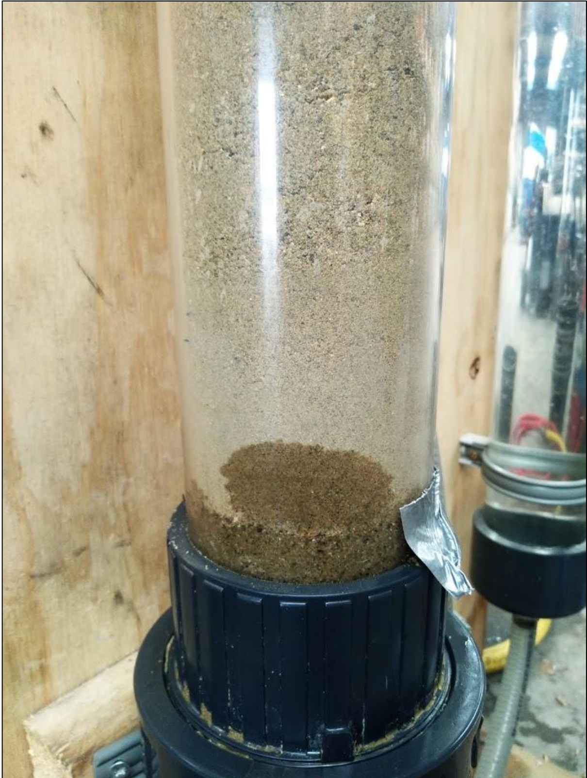
Figure 4.4.1 The onset of saturation of the sand column above the grouted soil. Top of the duct tape indicates the top of the grouted soil. The uneven saturation indicates the presence of preferential flow paths.
