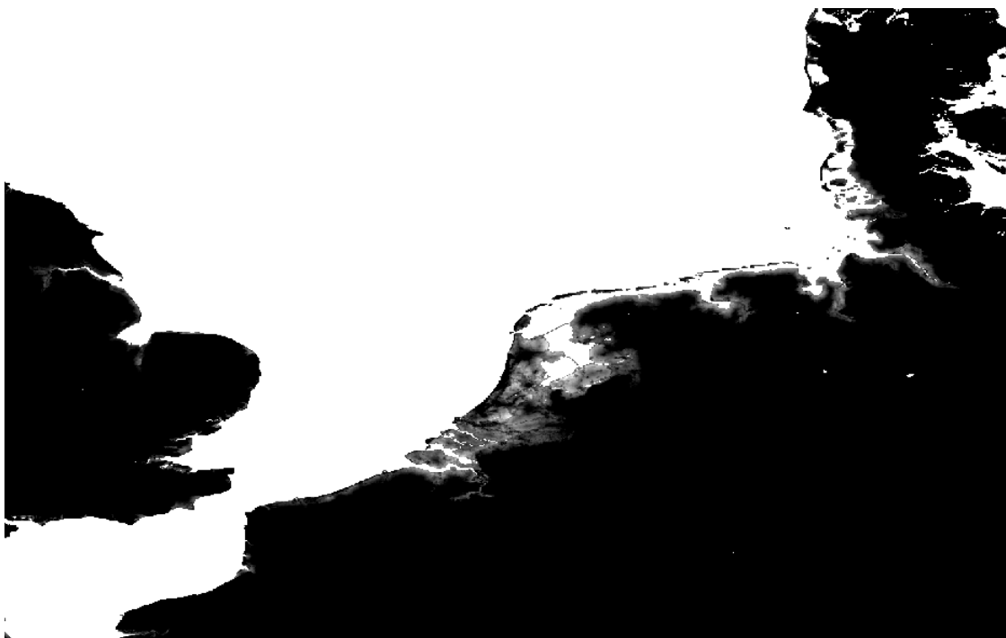
Figure 10: Example of flood statistic raster map. This section of the map shows the flood inundation from black (0 meters), to white (10 meters), of a 1000-year coastal flood. Data come from the WRI Aqueduct model (Ward et al., 2020).
