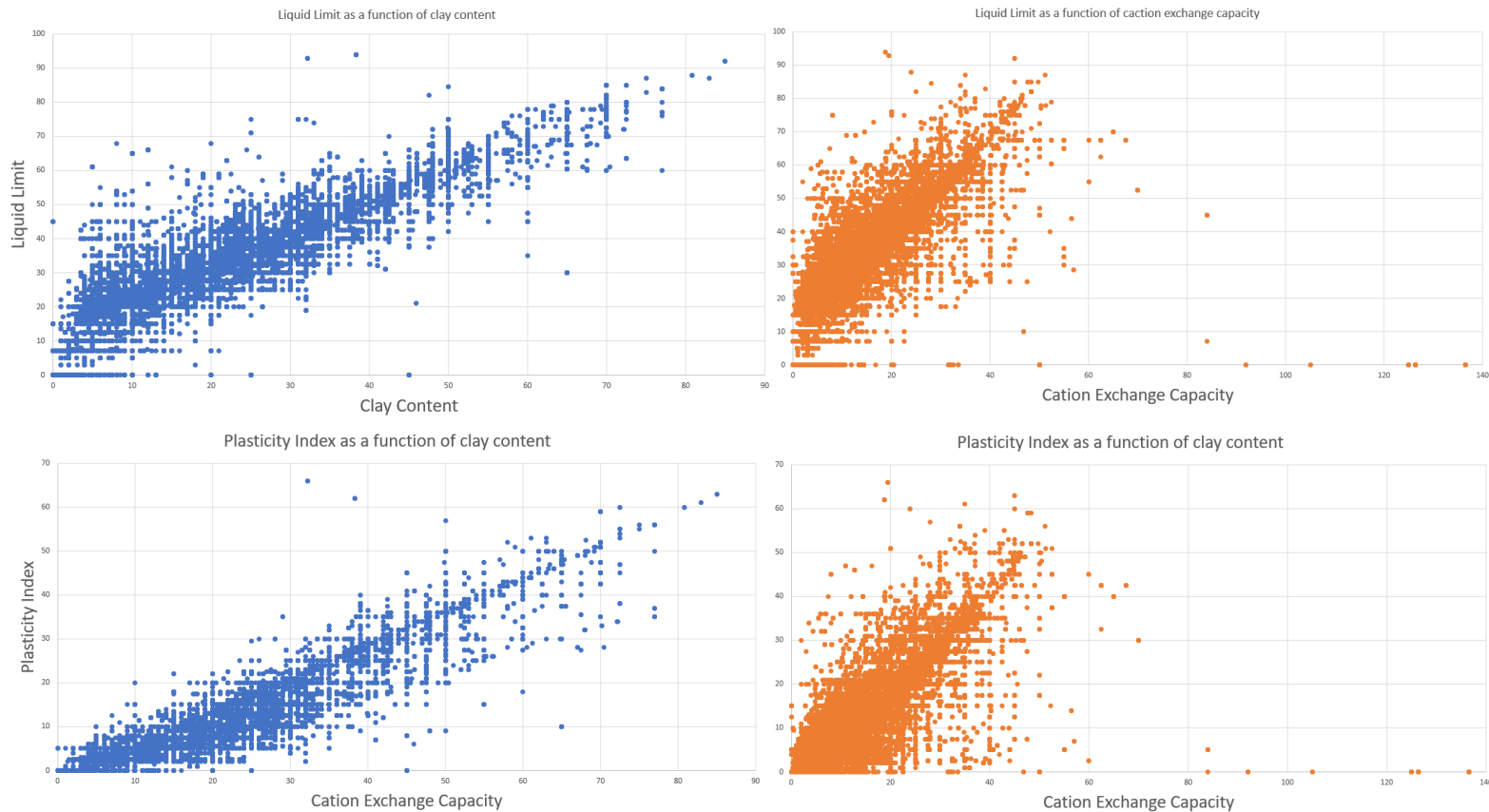
Figure 3.5: scatter plots of liquid limit and plasticity index as a function of clay and cation exchange capacity
